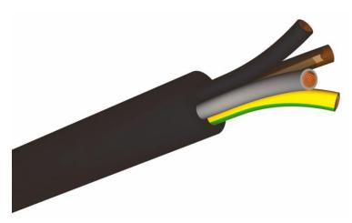
Construction: Flexible bare copper conductors according to CEI 20-29 Class 5 and DIN-VDE 0295
