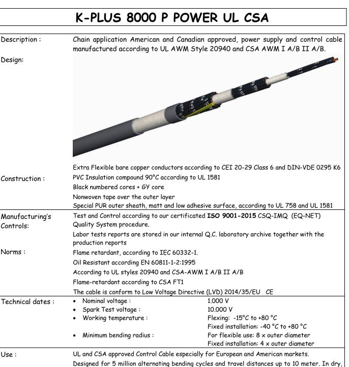
damp or wet interiors. Suitable for use in measuring, control and regulating circuits so as in
